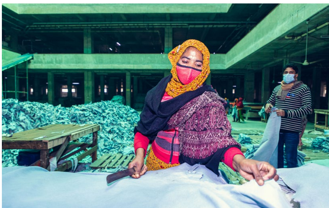
Female worker removes unnecessary substances (meat, fat etc.) from skin.
